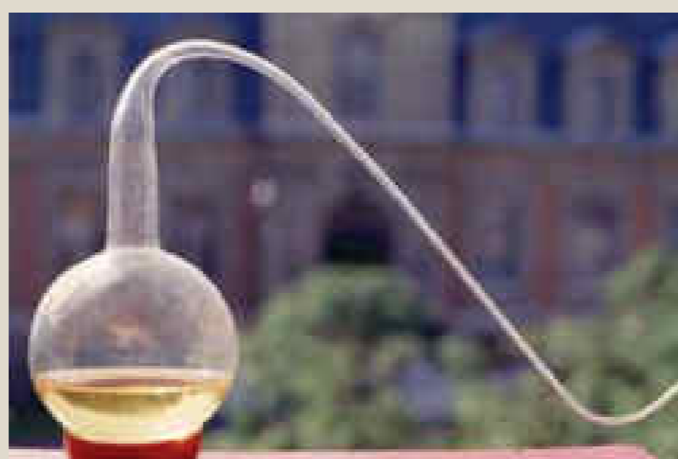
Swan neck flask used for Louis Pasteur's experiments challenging the spontaneous generation theory.
